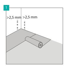
Lay Arbiton Multiprotec LVT Fastlay HD or Ewifoam Vinlay Rapid HD in a direction perpendicular to the direction in which panels are laid, maintaining the 2.5 mm wall expansion joint. The neighbouring underlay ribbons must be fitted to each other, without leaving any unnecessary space.
