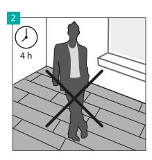
If the panels are installed to the substrate using an adhesive, heavy objects may be placed only after 24 hours from the gluing process, and the floor may be walked on gently after 4 hours from the gluing process.
