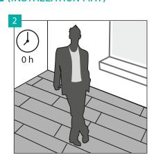
In the case of installation of the panels to the installation mat ("FASTLAY"), heavy objects may be placed already after 2 hours from the installation process, and the floor may be walked on directly after the installation.
